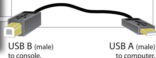
**Step 3:** Plug in the USB A into the computer.
