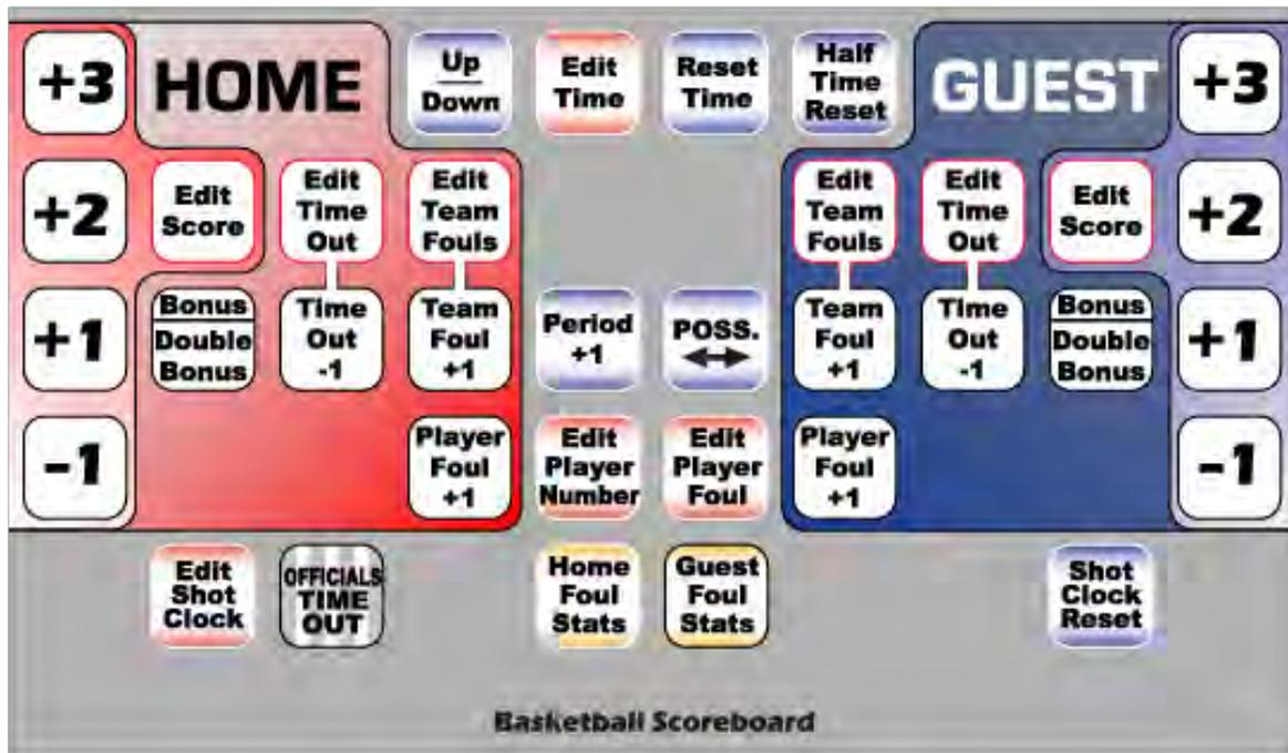
Basketball Scoreboard Slipsheet. This slipsheet can control all basketball scoreboards. For basic boards (8206,8208,8209), the reverse side of slipsheet may be used, eliminating many of the keys shown.
