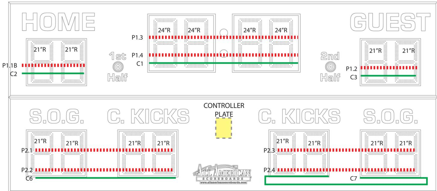
Power Supply Outputs (Full Brightness & Full Digits): P1.1 ≈ 3.26A P1.2 ≈ 2.60A P1.3 ≈ 2.83A P1.4 ≈ 2.83A
