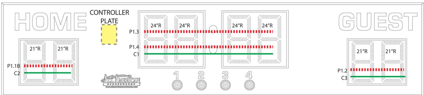
Power Supply Outputs (Full Brightness & Full Digits): P1.1 ≈ 3.42A P1.2 ≈ 2.60A P1.3 ≈ 2.81A P1.4 ≈ 2.81A
