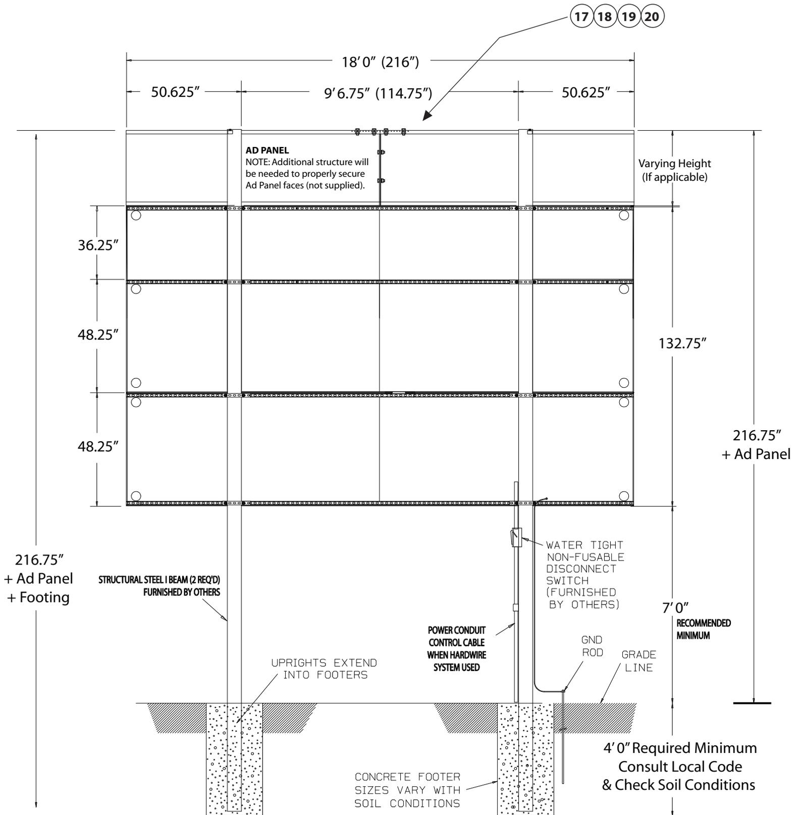
**NOTE: Foundation shown for illustration only. Actual foundation needs to meet national and local building codes. Sites must be surveyed by qualified engineer. All measurements are for reference only.**
