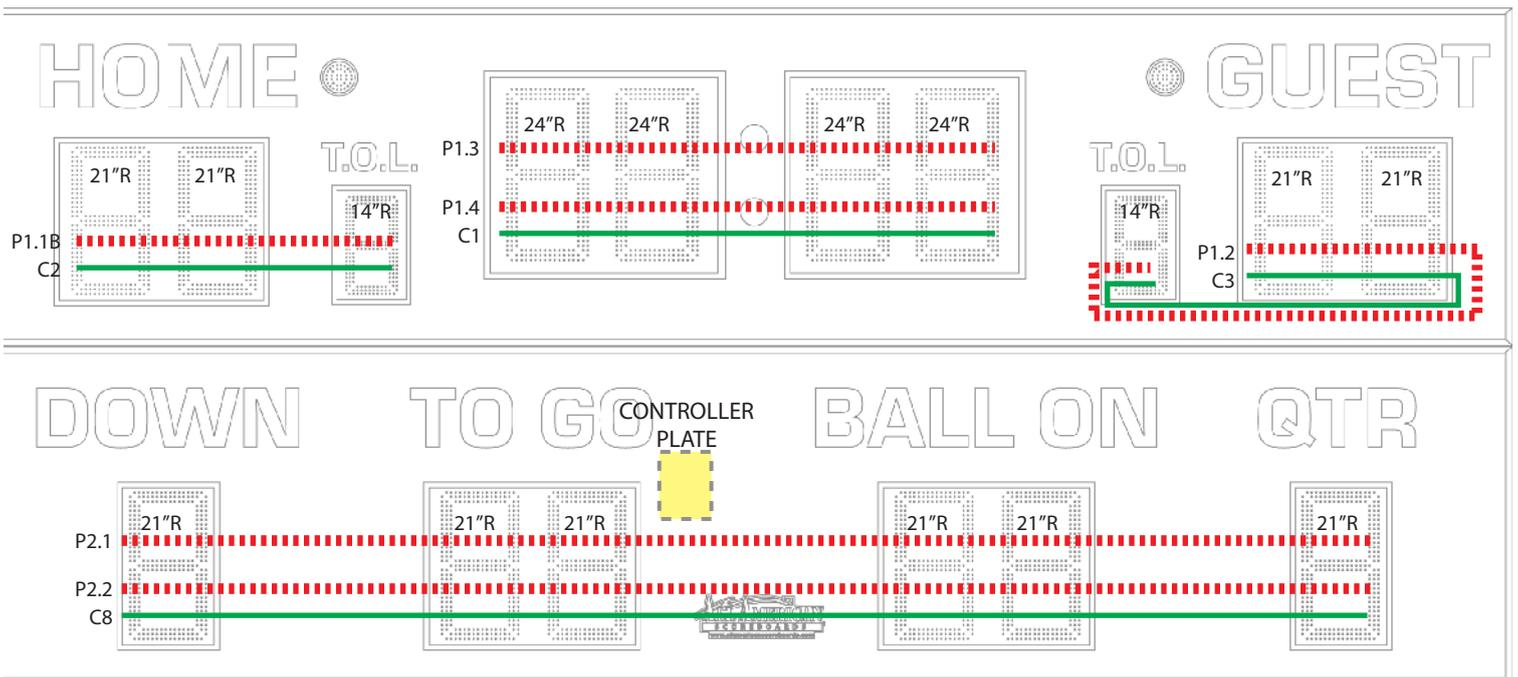
Power Supply Outputs (Full Brightness & Full Digits): P1.1 ≈ 4.23A P1.2 ≈ 2.81A P1.3 ≈ 2.81A P1.4 ≈ 3.57A
