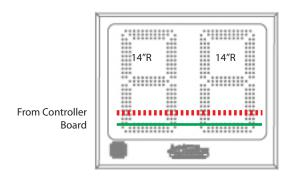
Power Supply Outputs (Full Brightness & Full Digits): P1.1≈2.44A (2.57 with 450N Horn)
