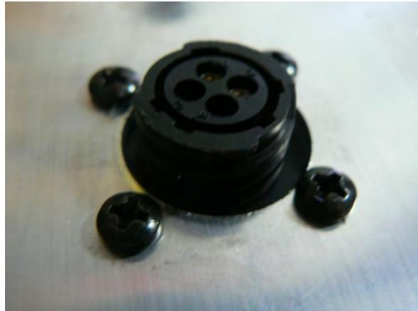
**12. Using (4) of the self tapping screws provided, mount power supply with DC connector no more than 15" away from connector on shotclock.**
