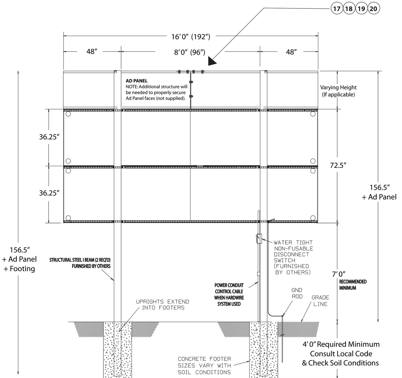
**NOTE: Foundation shown for illustration only. Actual foundation needs to meet national and local building codes. Sites must be surveyed by qualified engineer. All measurements are for reference only.**
