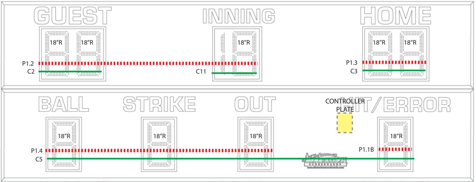
Power Supply Outputs (Full Brightness & Full Digits): P1.1 ≈ 1.69A P1.2 ≈ 3.92A P1.3 ≈ 2.38A P1.4 ≈ 3.57A
