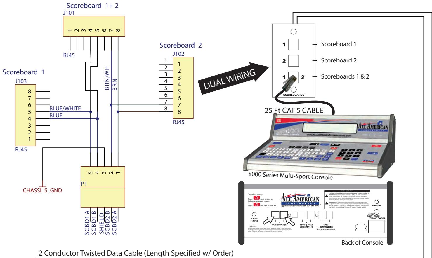
2 Conductor Twisted Data Cable (Length Specified w/ Order)
