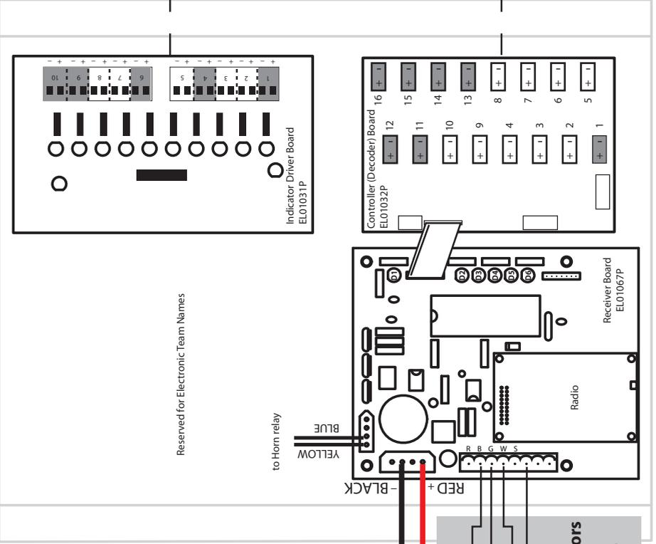
"C" refers to controller board output. If Indicator are used, C4 data will go to the Indicator Driver Board and then to the digit(s).
