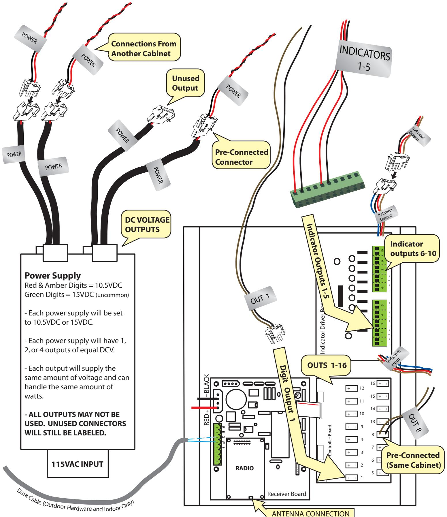
**Sample connections - connections and hardware will vary depending on specific scoreboard.**
